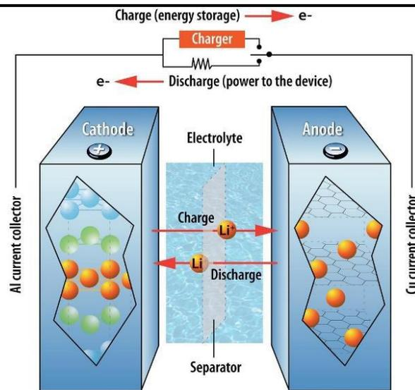
Figure 1. How the lithium-ion battery (LIB) works.
