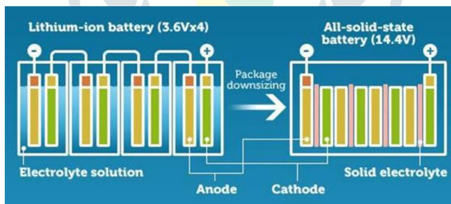
Figure 2. Diagram of (a) Lithium-ion Battery; (b) All Solid-State Battery [1].
