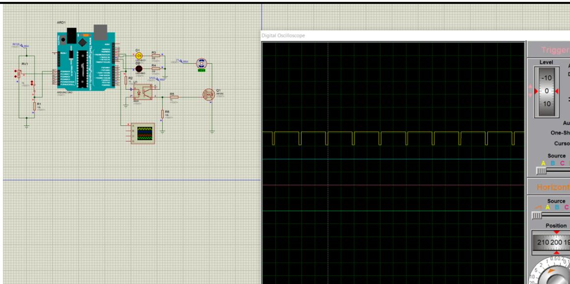
Fig.6. PWM is directly proportional to accelerator if pot value is less then duty cycle value is also less.
