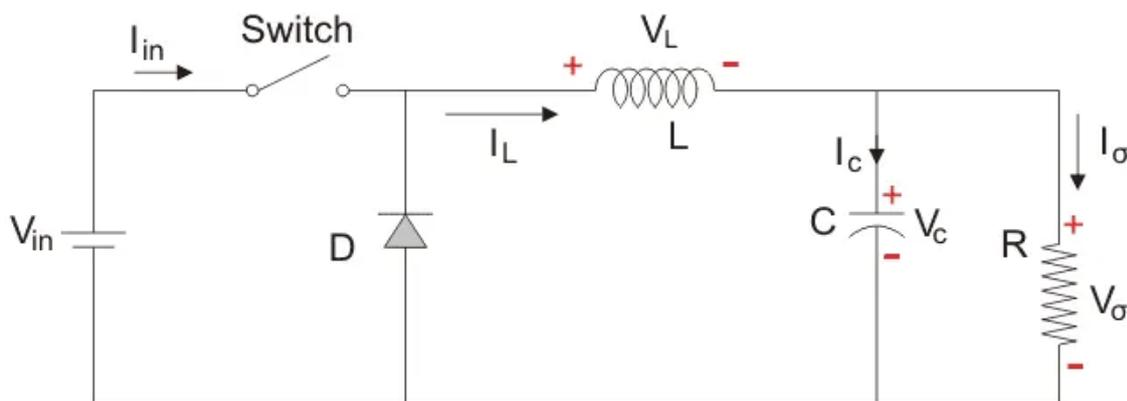
Figure 4: Mode II of buck converter
