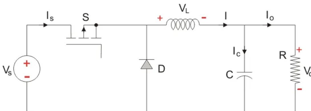
**Figure 2: DC – DC Buck Converter**
