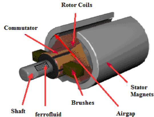
Fig.4. PMDC motor Structure
