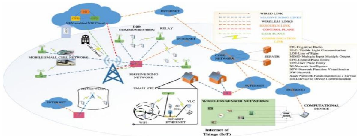
**Fig. 1: Fifth Generation Mobile Technology Network Architecture [Research gate].**
