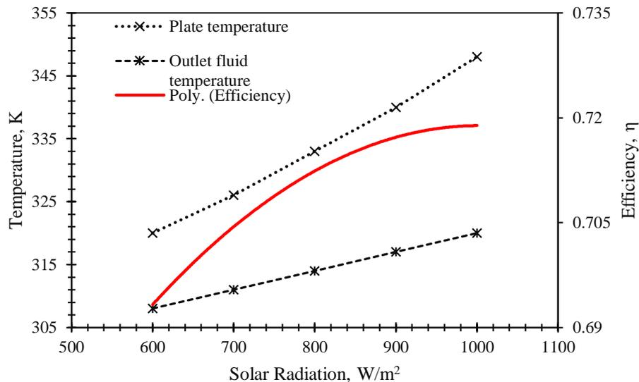
**Fig.2. Variation of Plate Temperature, Output Temperature and Efficiency**
