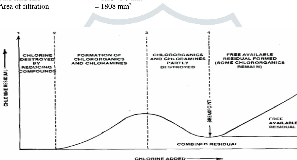
Fig. 1: Theory Of Break Point Chlorination
