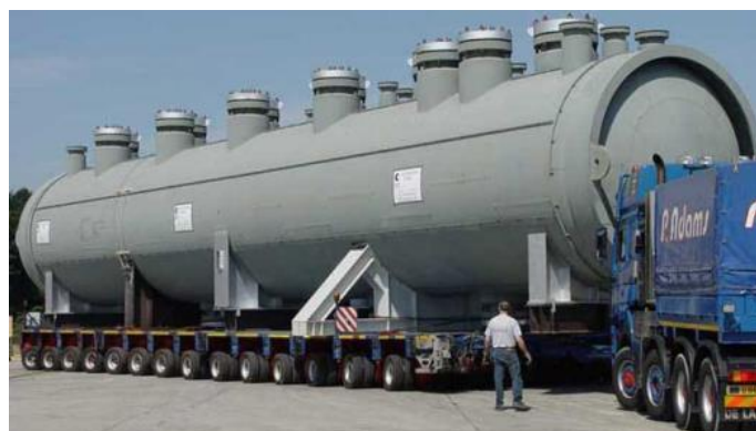
Figure 6 (a) Titanium Clad pressure vessel (Picture is the property of Coek Engineering NV, Lessel 13-2440, Belgium)
