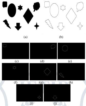
The fig (a) shows the original image. This image is processed using canny edge detector to get the image in fig (b) which is a binary image. The resulting binary image is provided as input to the blob extraction algorithm which extracts all the objects from the image as shown above.
