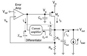
Fig 2 LDO topology with differentiator for fast transient path.
