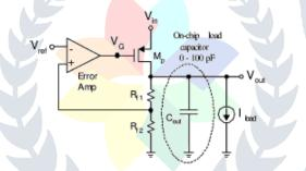
Fig 1 : Basic LDO voltage regulator.
