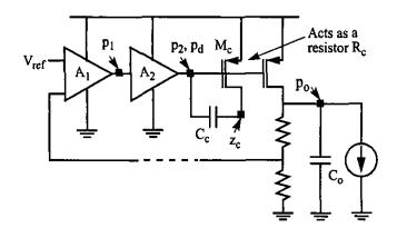
Fig 5: Pole-zero tracking frequency compensation for low dropout regulator.
