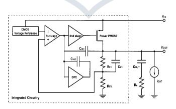
Fig 4: A capacitor-free CMOS low-dropout regulator with damping-factor-control frequency compensation *4. Pole-zero tracking frequency compensation*
