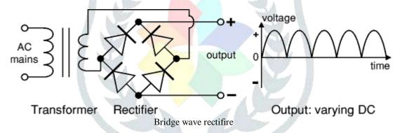
In this only two diodes are activated at a time i.e. D1 and D3 activate for positive cycle and D2 and D4 activates for negative half cycle.D2 and D4 convert negative cycle to positive cycle as it as negative supply and negative cycle as positive cycle at its output.
