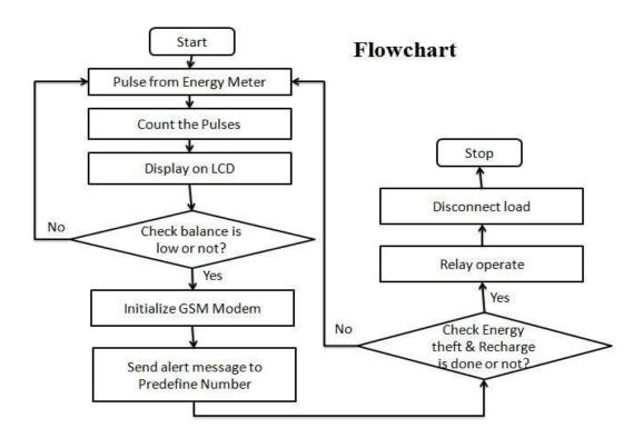
Above flow chart state that energy meter can generate the pulses and this generated pulses counted on LCD. This pulses is converted into watt and this watt displayed on LCD as per used by consumer or load. Then after controller check the balance if balance is higher than predefined rupees then no to worry but balance is low than predefined rupees than GSM operate and start to work and sending the alert message to the consumer about the recharge the energy meter balance.
