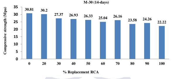
Fig 7: 14-days Compressive strength of M-30 mix concrete with different replacement level of recycled aggregate.
