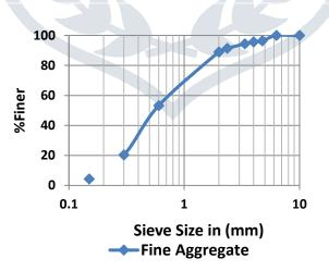
Fig 2: Particle Size Distribution of Fine Aggregate (Natural Sand)
