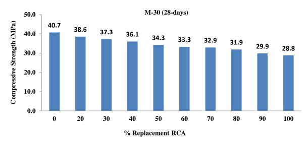
Fig 9: 28-days Compressive strength of M-30 mix concrete with different replacement level of recycled aggregate.
