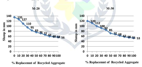
Fig. 3 Slump test result for Mix- M-20 & M-30
