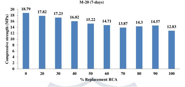
Fig 4: 7-days Compressive strength of M-20 mix concrete with different replacement level of recycled aggregate.
