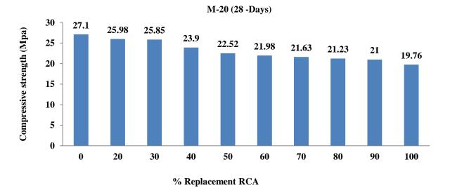
Fig 8: 28-days Compressive strength of M-20 mix concrete with different replacement level of recycled aggregate
