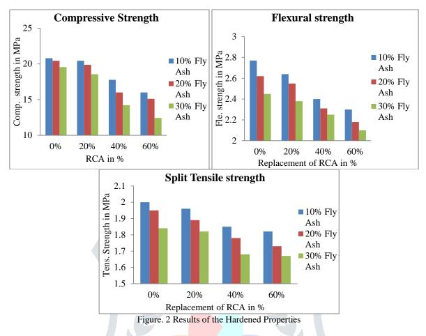
Obtained results of each tests are given below in tabular form for water cement ratio 0.50.
