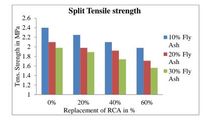
Figure. 4 Results of the Hardened Properties
