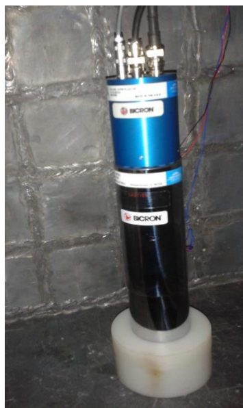
Figure 1: 2" x 2" NaI(Tl) Gamma ray detector.
