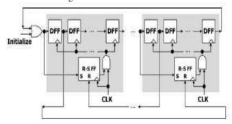
Figure 3 Ring counter with RS flip-flop
