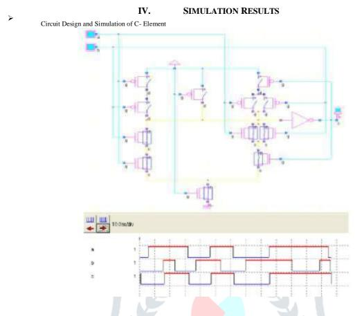
Design and Simulation of Proposed Ring Counter of Double edge triggered Flip Flop with Clock Gated by C-Elements
