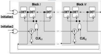
Figure 5 Diagram of Ring Counter with Clock gated by C-elements
