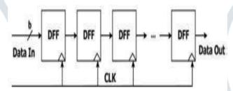
Figure 1 Delay Buffer implemented by Shift Register
