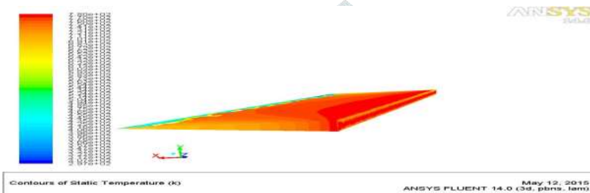
Figure 9:- Heat distribution on triangular fins
