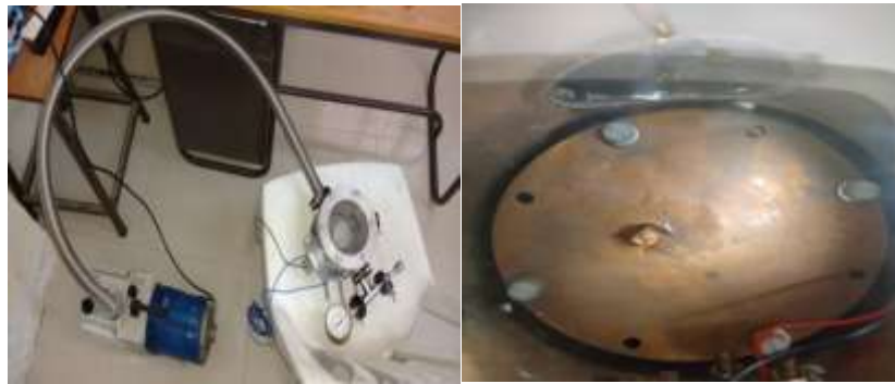
a. Degasification Set-up b. Component in vacuum chamber
