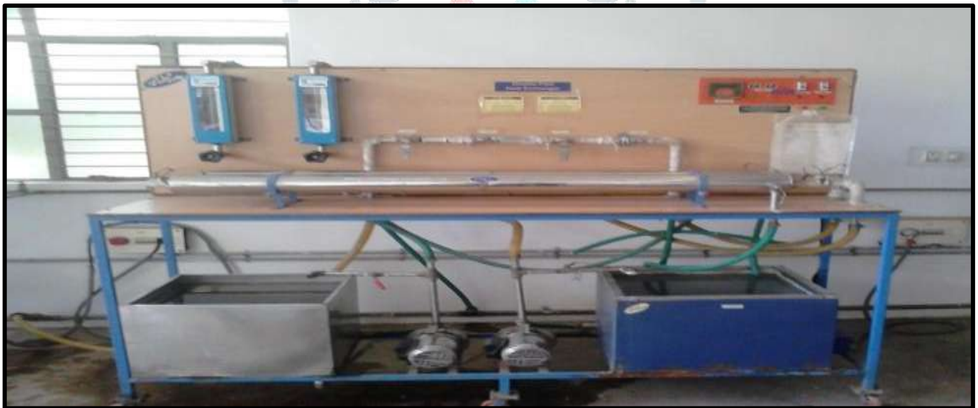
FIGURE 2 : Experimental Setup of Double Pipe Heat Exchanger Apparatus
