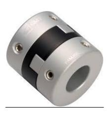
di = internal diameter = 16 mm Dh = Hub diameter = 2di  $=2 \times 16$ =32 mmDh≈50 mm Length of hub Lh = (2 to 2.5) di= 2.5 x di $=2.5 \times 16$ =40 mm≈50 Failure of hub Considering shear failure (t) Material C.I.SAE 30 Sys = 98, F.O.S = 3 $t max = 98/3 = 32.66 \text{ N/mm}^2$  $t = P/A = 540/(\pi \times (50^2 - 16^2)/4)$  $t = 0.306 \text{ N/mm}^2$  $t \text{ max} = 32.66 > 0.306 \text{ N/mm}^2$ So our design of hub is safe.
