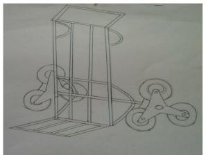
II. When a man will pull the handle of truck, the wheel 'A' will fix in corner which is made by the ground and step 1. After that when man will pull handle again the wheel 'B' will fixed in corner which is made by step 1 and step 2. Again man pull the truck, the wheel 'C' will fixed to the position at corner of step 2 & step 3 and so on. This working is repeated again and again while climbing on stairs vice versa.
