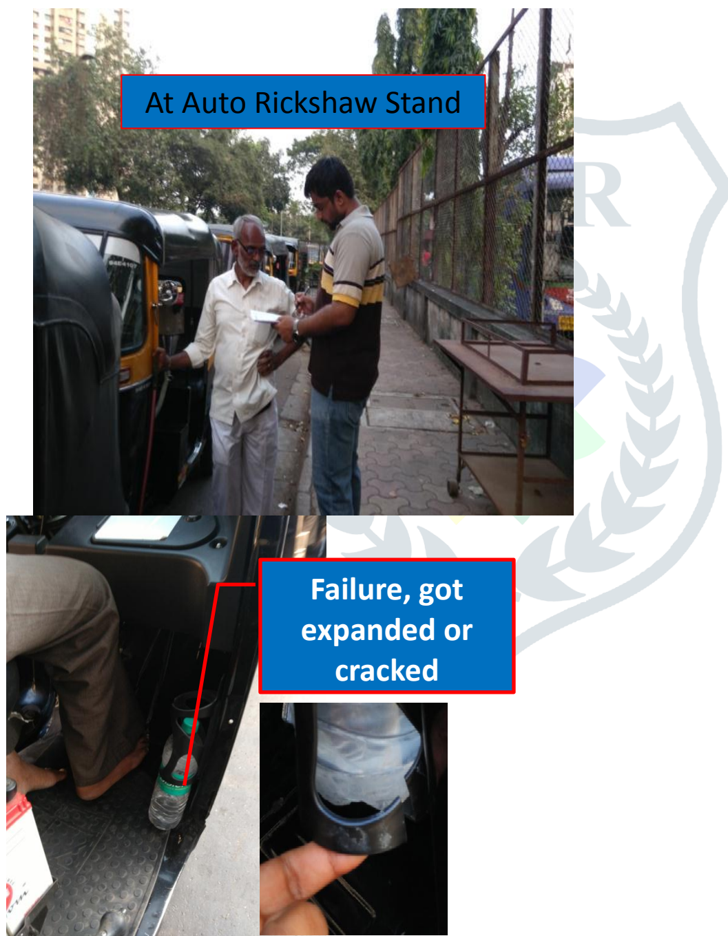
Fig 1. Failure of Bottle Holder
