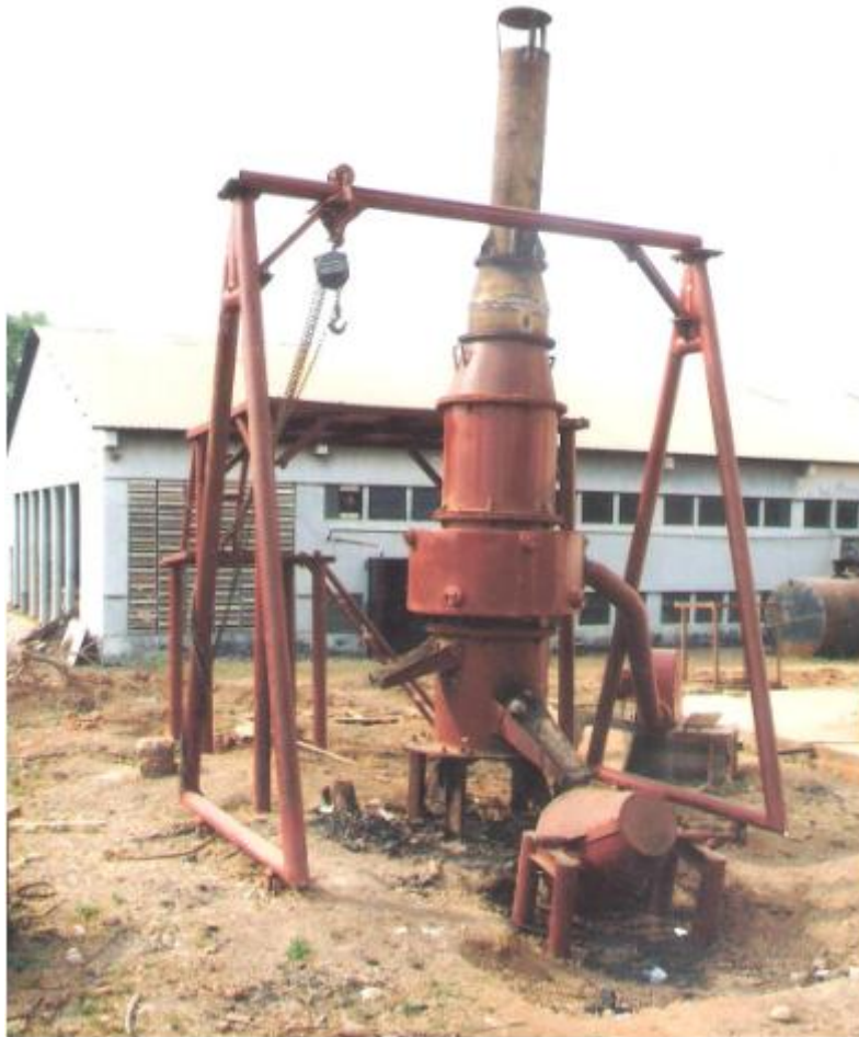
Fig2 . pictorial view of a cupola furnace in use SEDI ,Enugu
