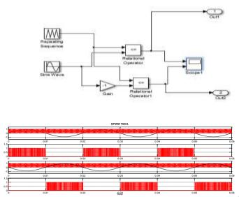
Fig.5. Simulation of SPWM Technique [11]-[12]
