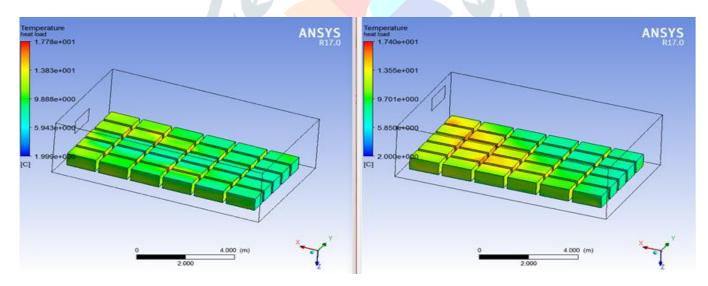
Fig -17 Loading condition temperature distribution in vegetable
