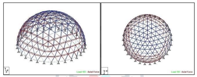
Figure 4 Isometric view and top view of axial force diagram for Model11-6-10
