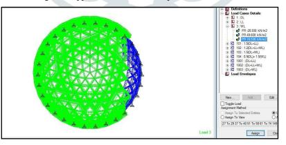
Figure 3 Application of Wind load pressure Pz<sub>3</sub>
