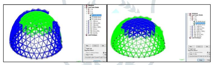
Figure 2 Application of Wind load pressure Pz1 and Pz2
