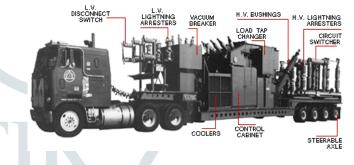
Fig. - Component of mobile transformer
