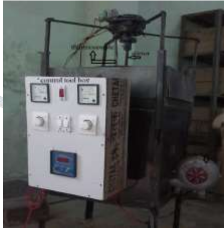
Fig. 2 Experimental set-up of Stir casting
