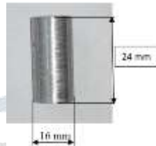
Fig. 6 Specimen configuration and size for compressive strength test
