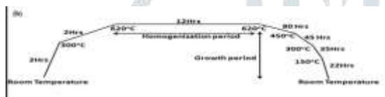
Fig 4- (a) Procedure to grow single crystal of Bismuth Telluride [4]. (b) Temperature profile of the furnace.
