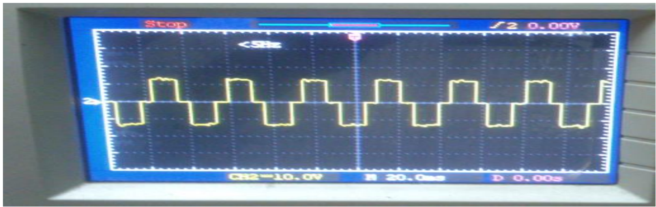
Figure 8. Output voltage of three level inverter system
