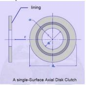
Now the torque that can be transmitted by this elemental are is equal to the frictional force times the moment arm about the axis that is the radius 'r' i.e.
