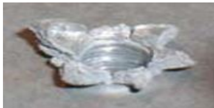
Fig. 1 Friction drilling cast Al part with flower shape bushing
