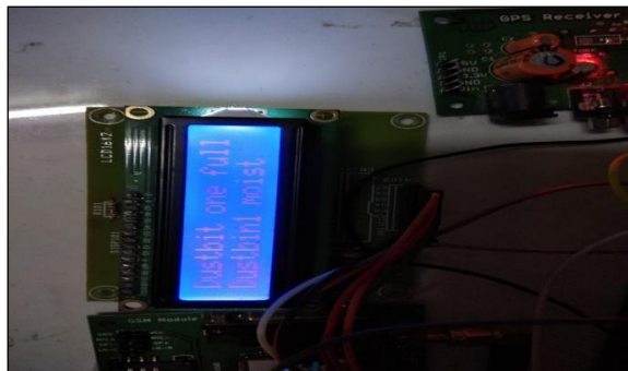
Fig 10. Detection of moisture content in the dustbin
