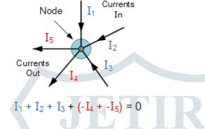
Here, the three currents entering the node,  $I_1$ ,  $I_2$ ,  $I_3$  are all positive in value and the two currents leaving the node,  $I_4$  and  $I_5$  are negative in value. Then this means we can also rewrite the equation as;
