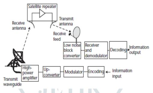
Figure [3]: Critical elements of the satellite link.
