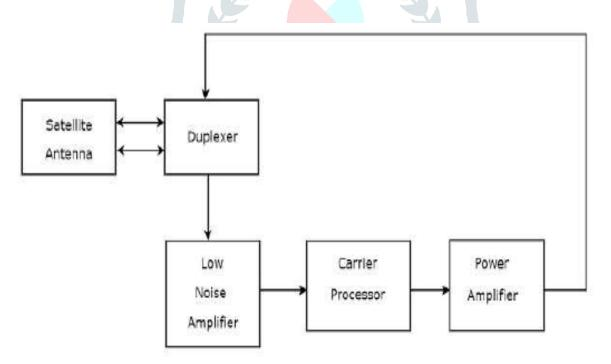
Fig. [1]: The block diagram of transponder
