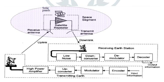
Figure[2]: Basic communications satellite components
