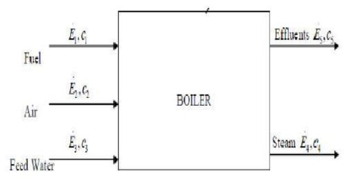
Fig. 1. Inlet and outlet Streams for a boiler system
