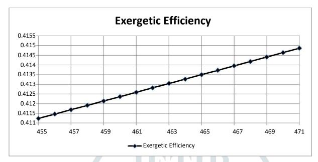
Fig. 2 Effect of feed water temperature on exergetic efficiency of the boiler system
