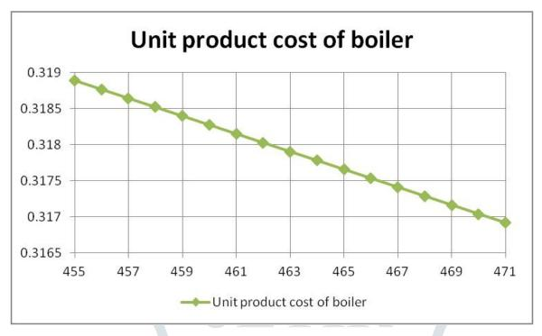
Fig. 4 Effect of feed water temperature on the unit product cost of the boiler system
