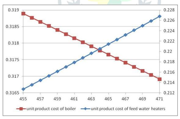
Fig. 5 Combined effect of feed water temperature on unit product cost of boiler and feed water heaters
