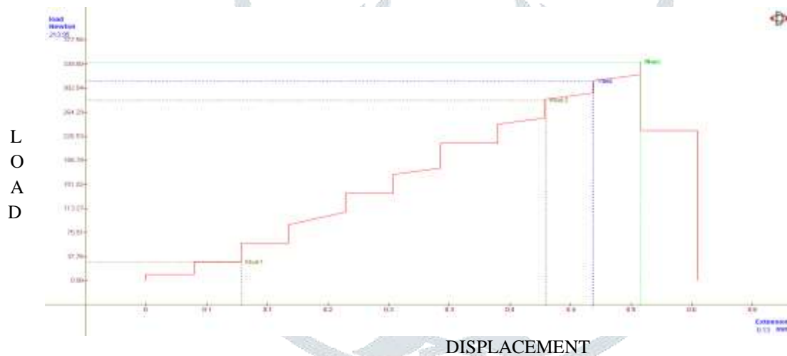
Graph:- 5.2 Load vs displacement graph of 50mm fiber size tensile tested specimen
