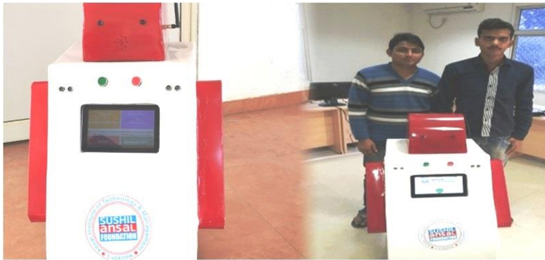
FIGURE 1: A HUMANOID ROBOT HAS BEEN DEVELOPED FOR THE ADVANCEMENT OF THE INSTITUTE. THE ROBOT WILL TELL THE ASKED INFORMATION ABOUT THE INSTITUTE IN VOICE. THE ROBOT WILL BE SELF-DRIVEN; IT WILL FIND ITS PATH BY ITSELF.
