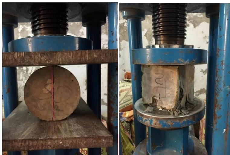
Figure 3 Compressive Strength test Machine with Specimen
