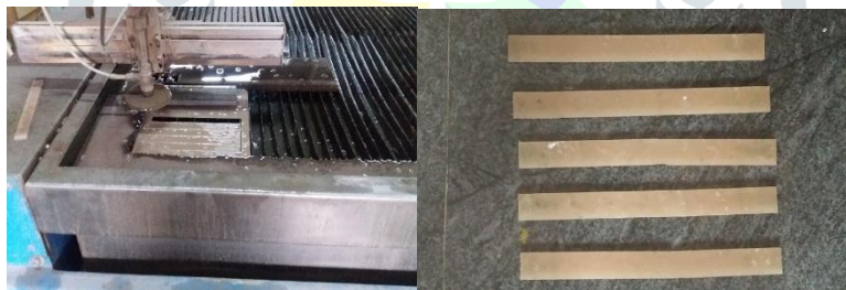
Figure No.1 Cutting of specimens using water jet machine
