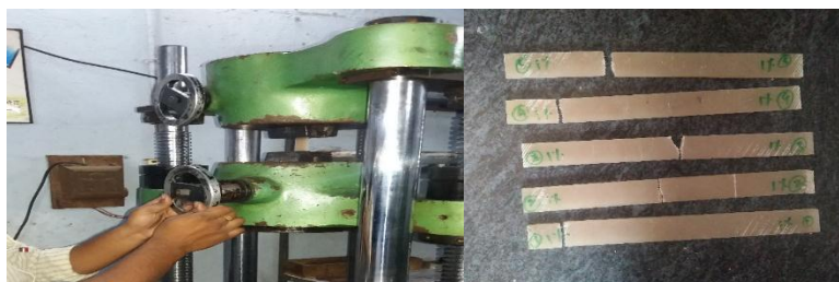
Figure No. 2 Testing of tensile specimens
