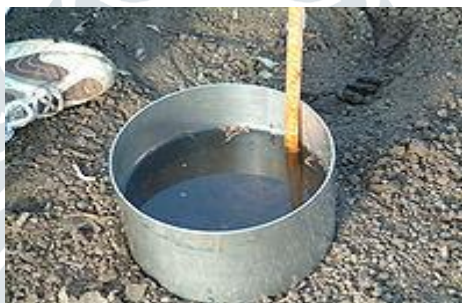
Figure 3 Single Ring Infiltration
