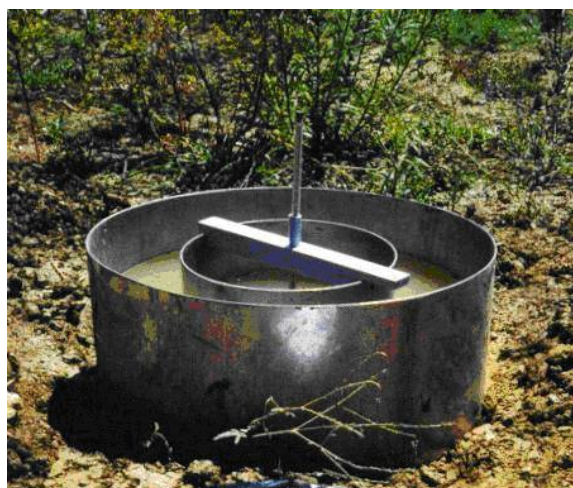
Figure 4 Double Ring Infiltration
