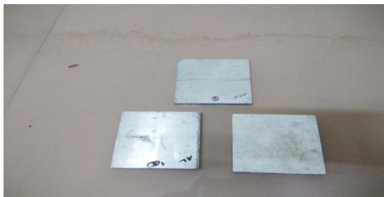
Fig. Specimens as per ASTM B117 Standard
