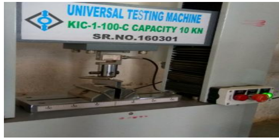
Figure no 4 ILSS test set up
