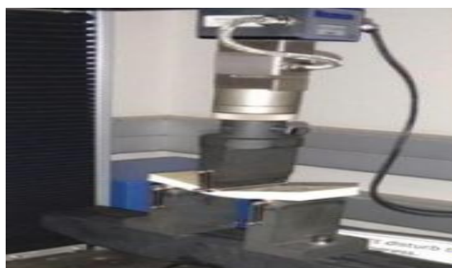
Figure no 3 Flexural test set up
