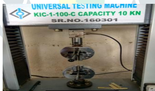
Figure no 2 Tensile test set up
