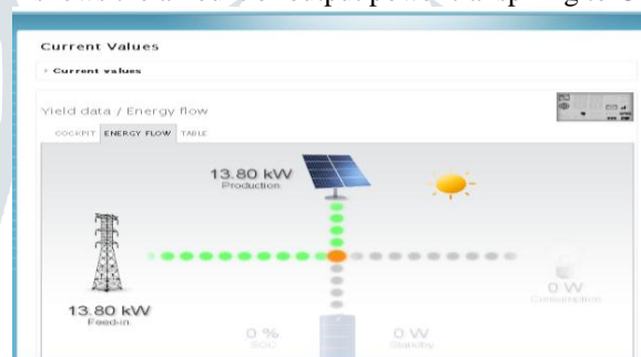
Figure 11 Power transpiring to grid from solar plant
