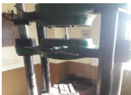
Fig. 7 Specimen Loaded in UTM
