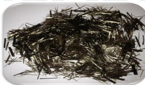
Fig. 2 Chopped Basalt Fiber
