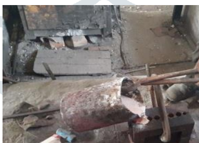
Fig. 3 Pouring Hot Mixture in Mould
