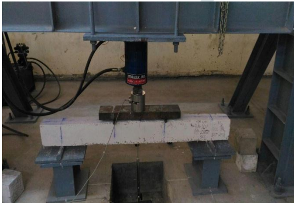
Fig 4.1 SCC control Beam
