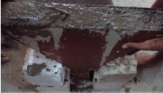
Fig 3.4 V-Funnel test on fresh concrete.
