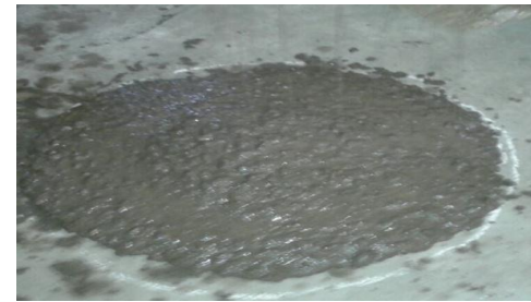
Fig 3.2 Slump Flow test on fresh concrete.
