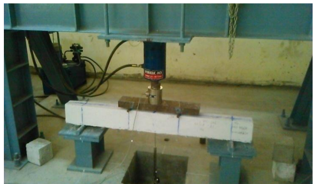
Fig 3.7 Loading Frame Setup
