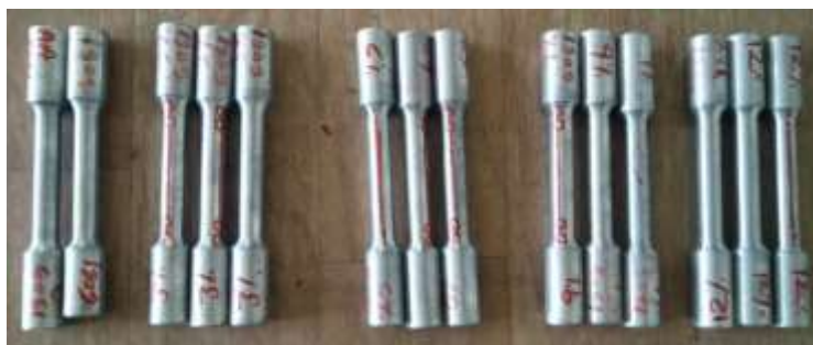
Figure 5.2 Machined Tensile test specimens as per ASTM Standards
