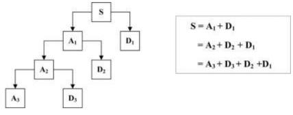
Fig. 4. Three-level decomposition of a signal 'S'.
