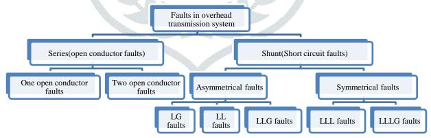
Fig. 1. Classification of faults.
