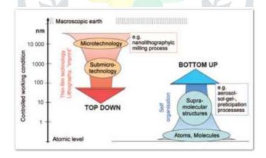
Methods of nanoparticle production (Source: https://www.nanowerk.com/how\_nanoparticles\_are\_made.php)
