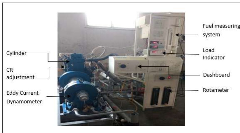
Fig. 1: Actual engine setup of 4 stroke VCR testing
