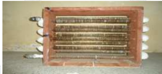
Figure 2.2 With fin heat exchanger
