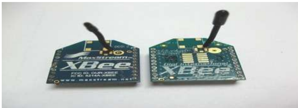
Left is XBee Series 1, Right is XBee Series 2 Point to point two way communications
