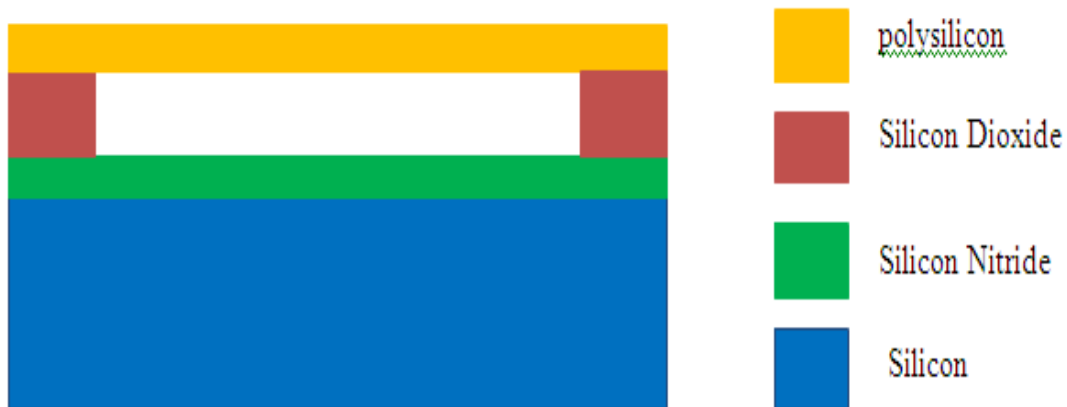
Fig 4.2 schematic of a single cell of CMUT
